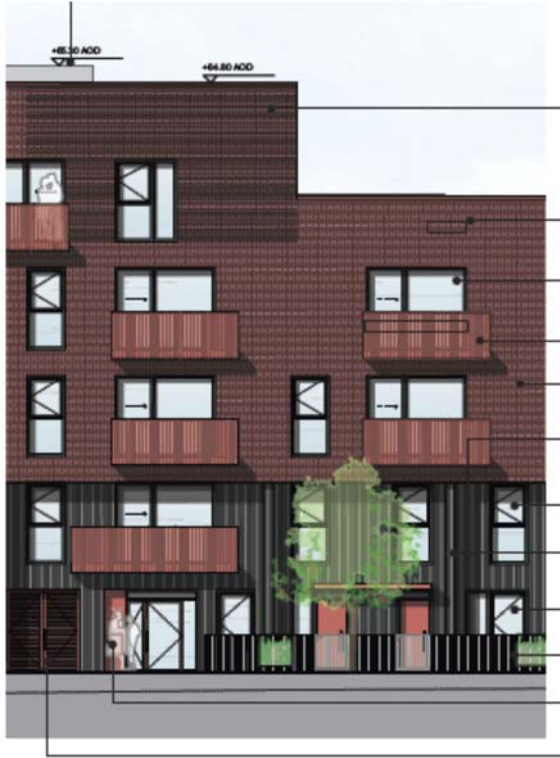
Image 8: Typical elevation of Block D showing the communal entrance and the treatment of the two storey maisonette homes
